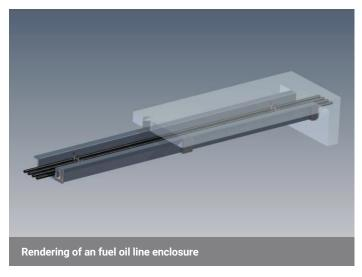
VaughanAir's '2HR' enclosures are available with an E119 listed fire rating of 2 hours with a built-in containment provision designed to protect fuel oil lines in accordance with New York City Building Code.
